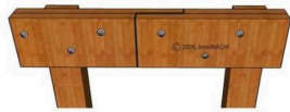
The illustration above depicts a butt joint or splice improperly located within a girder span. Butt joints in a girder span are generally not permitted unless specially engineered. A butt joint or splice should be positioned to land at the posts.
